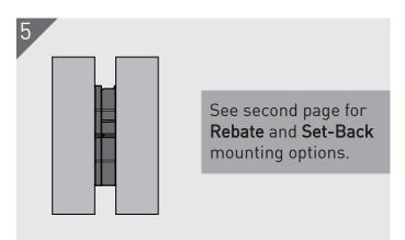
When assembled, the substrates will be separated by the thickness of the engaged Clip 50.
