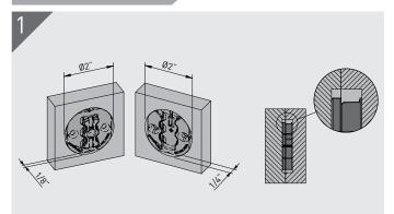
**Part Rebate** - each substrate mounting face is rebating as shown. Ensure sufficient screw embedment in substrate.
