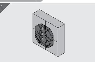
Mark center lines, vertical and horizontal, on both substrates. Flush mounting requires no additional preparation. Line the notches in each component (Hook shown here) with the center lines. **Mark-Out Template** can also be used.
