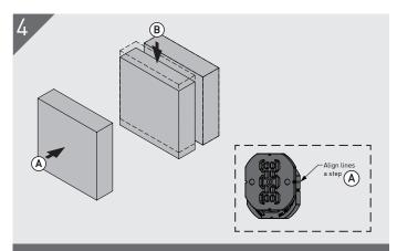
Assemble the joint remembering the Clip 50 only needs to travel 1 pitch for full engagement. Alignment lines are deigned into the parts to help with assembly.
