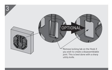
Prior to assembly, establish whether the joint is to be permanent or disassemblable.
