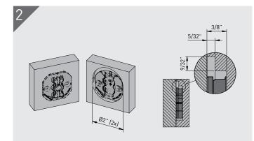
**Full Rebate** - 1 of the substrate mounting faces is rebating the full depth as shown. Ensure sufficient screw embedment in substrate.
