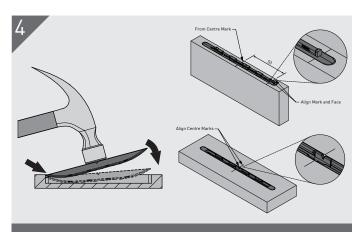
To aid in the installation of the Hook and Key, start by inserting one end in the slot when use a hammer or mallet to tap the component into place.
