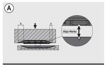
Note the offset of the lugs on the Key body, length X is larger than Y. Insert the Hook into the Key with the longer X end towards the face to be pushed during assembly.
