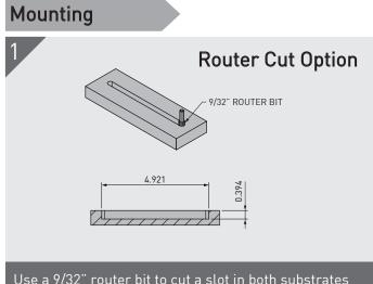
Use a 9/32" router bit to cut a slot in both substrates where the Hook and Key of the Mini 120 is to be mounted. Depth needs to be 0.394" for each.
