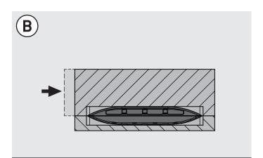
To complete the assembly push the end of the substrate (with X offset) until the Mini 120 is fully engaged.
