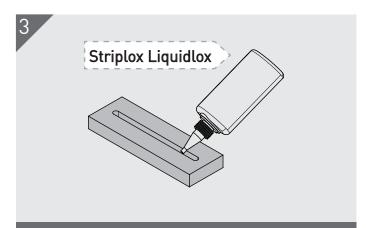
Apply Striplox Liquidlox 15 second cure adhesive to both sides of the slot in each substrate. *Visit* www.mcfeelys.com/installation or call 800-443-7937 to find out more about these products and Mark-Out Template.
