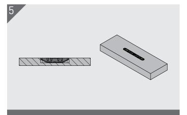
After glue is applied, insert Key and Hook into slot until flush with substrate. Allow to dry as per glue manufactures instructions.
