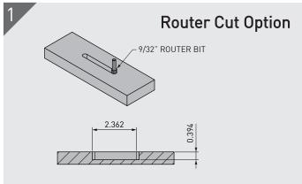
Use a 9/32" router bit to cut a slot in both substrates where the Hook and Key of the Mini 60 is to be mounted. Depth needs to be 0.394" for each.
