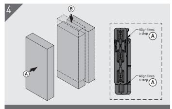
Assembly the joint remembering the Pro 23 only needs to travel 1 pitch for full engagement. Alignment lines are deigned into the parts to help with assembly.
