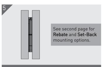
When assembled, the substrates with be separated by the thickness of the engaged Pro 23.
