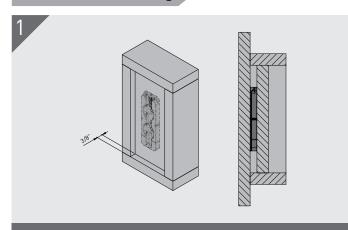
Setting back the mounting face of either the Hook (as shown) or Key by 3/8" results in a concealed joint without the need to cut rebates.
