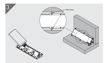
An alternative to marking screw locations is to apply glue to the mounting faces of the Hooks to aid with placement. Line up notches in the Hooks with the marked lines them press and hold the assembled 90D in place. Allow time for glue to dry.
