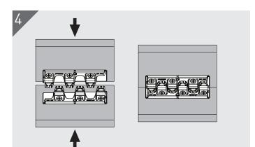
After all screws are in place, bring the two substrates together. The two sets of Hooks will self-align as shown.
