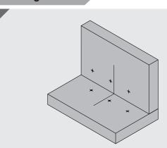
Mark center line on both substrates. The 90D 98 works on box joints (shown), t-section and mitered joints. Mark mounting screw centre points by measuring or with the aid of the **Mark-Out Template**.
