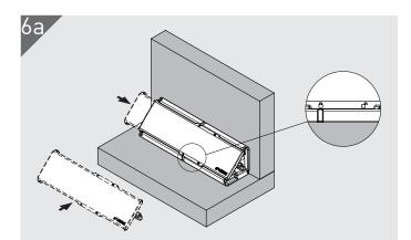
Install the Key remembering it only needs to travel 1 pitch for full engagement. Use the padlock symbol as a guide. The Key is also bidirectional and can be installed either end, see step 6b.
