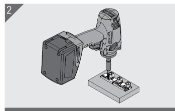
Fasten each Hook with 3 x 8G screws. Ensure sufficient screw embedment in substrate.
