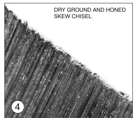
Photo 4 is after honing. Note the duller look of the honed surface and the root of the burr firmly in place.
