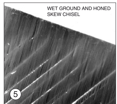
Photo 5. In this case the wet grinding method has been used in conjunction with the honing wheel. Note the clean polished edge.
